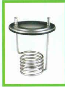
2610T Four Litre Temperature Control Coil •Stainless steel coil for use with 2610C or standard 4 litre CAC70 containers •Water circulated through helical coil cools media being processed •Comes complete with cover and gasket
