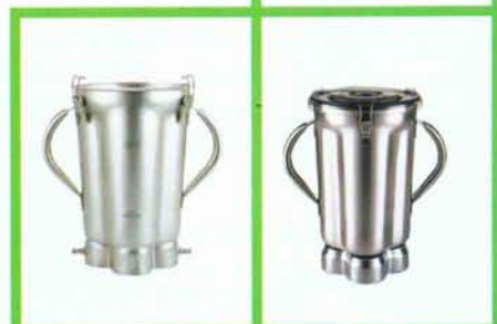
2610C Four Litre Cool Base Container •Four litre stainless steel container with jacketed base, allowing for water cooling of bearing during extended operation periods •Unit does not include lid or cover gasket
